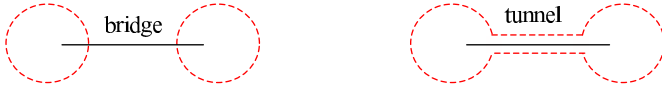
Fig. 2. Merge two chunk regions and boundary curves by digging a tunnel along a bridge
