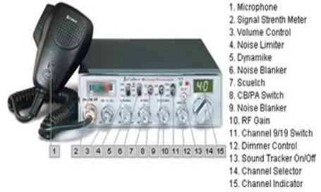
Fig. 2. A technical drawing of a cb radio
